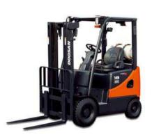
D15S / D18S-5 & D20SC-5 G15S / G18S-5 & G20SC-5 1,500kg 1,750kg 2,000kg Diesel, LP, Pneumatic Tire
