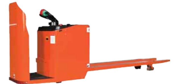
LEKH 20 Capacity: 2000 kg Fork length: 2350 mm Overall width: 760 mm
