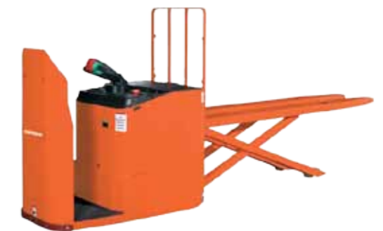
LEKX 20 Capacity: 2000 kg Lift height: 700 mm Fork length: 2350 mm Overall width: 795mm
