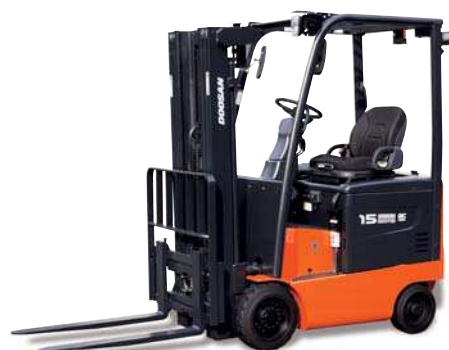
BC15S / BC18S-5 / BC20SC-5 1,500kg to 2,000kg Capacity 36/48 VOLT Cushion Tire
