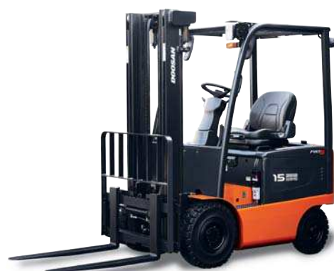
B15S / B18S-5 1,500kg to 2,000kg Capacity 48 VOLT Pneumatic Tire
